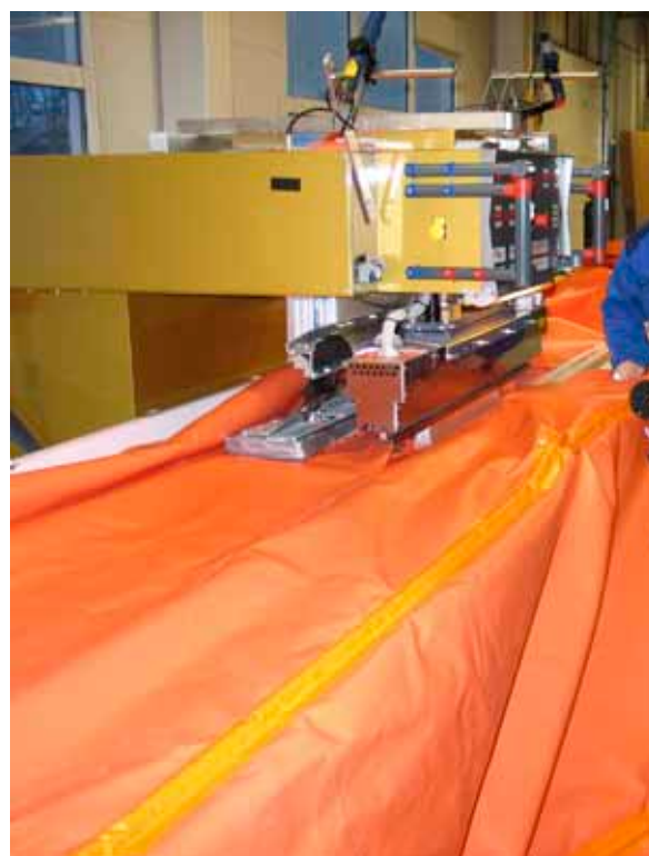
Figur 3.6. Plastsveisemaskin for store presenninger.
